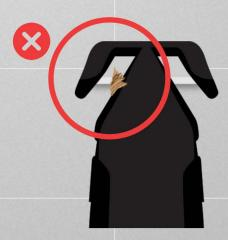
Clogged blades reduce operator cutting speed and introduce risk of injury when removing corrugate.
